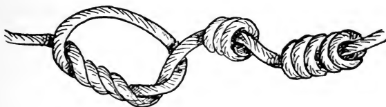
FIG. 69.—Three- and fivefold shortening.
